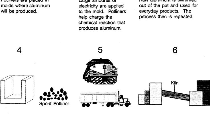
After 3 - 5 years the potliner becomes worn out and is removed and crushed into a gravel-like substance.
