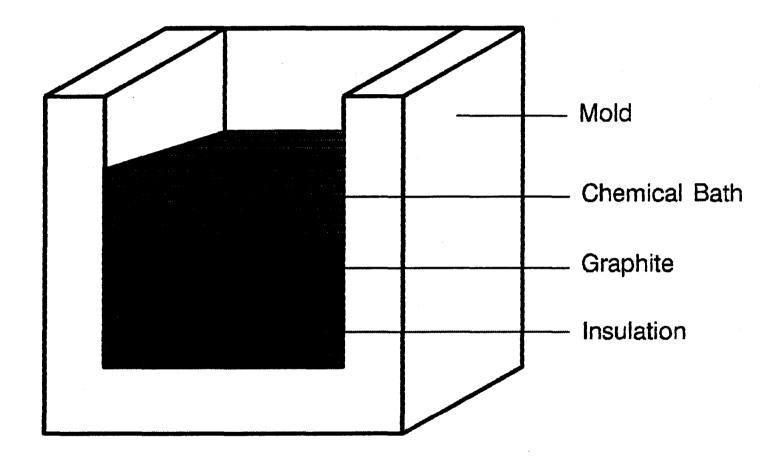
Potliners are made up of insulation material such as refractory brick covered with a graphite layer.
