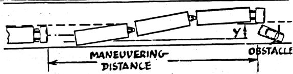
The "Crack-the-Whip Effect" is referred to as the "amplification Tatio or "amplification factor" in most engineering literature.
