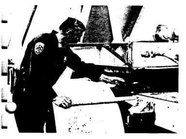
Check safety chains for adequate strength and proper hookup. The strength of a safety chain must be at least equal to the weight of the loaded trailer.
