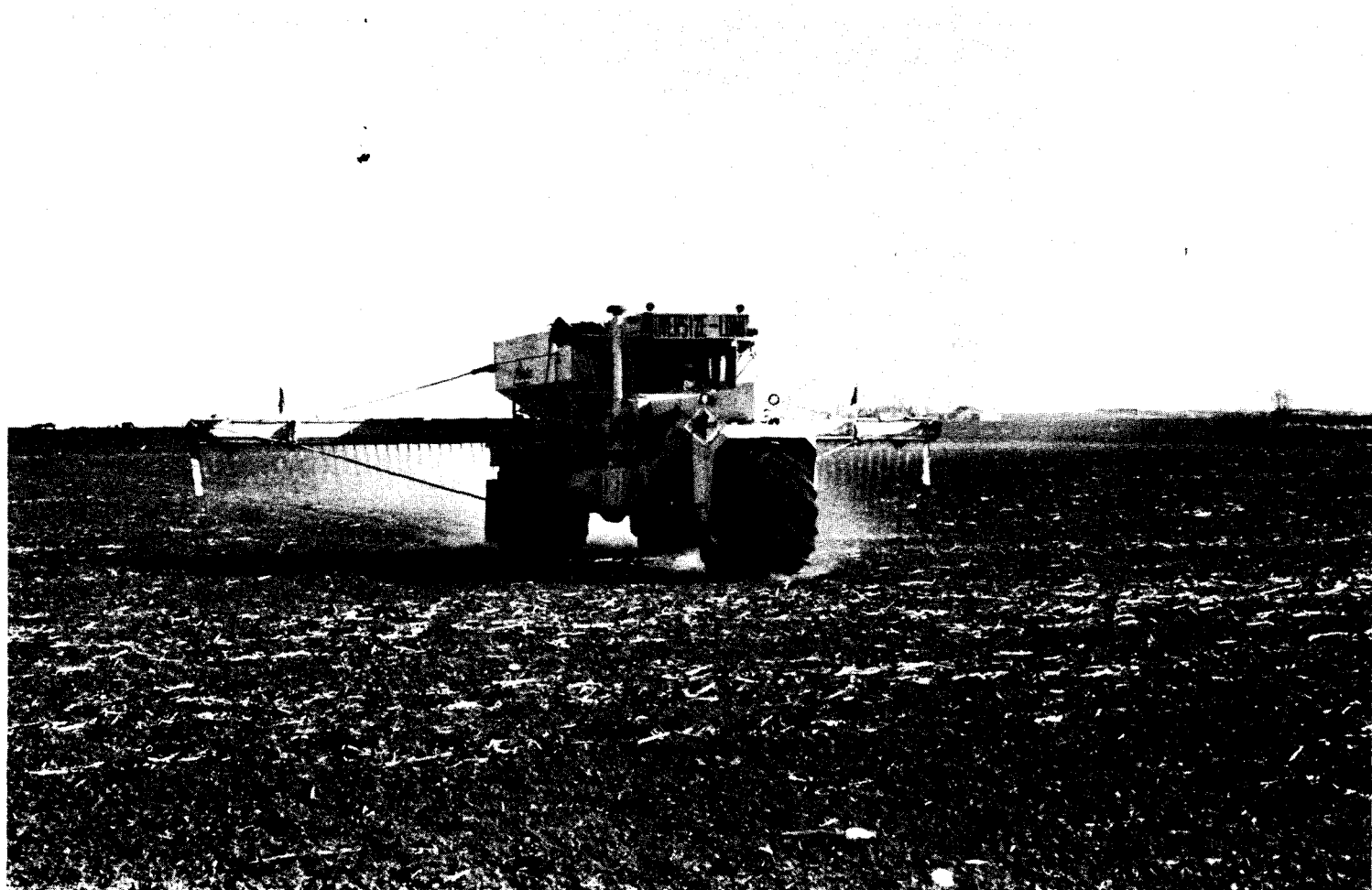
Fig. 16. Broadcast fertilizer equipment is used in some areas to apply liquid or dry fertilizer prior to planting.
