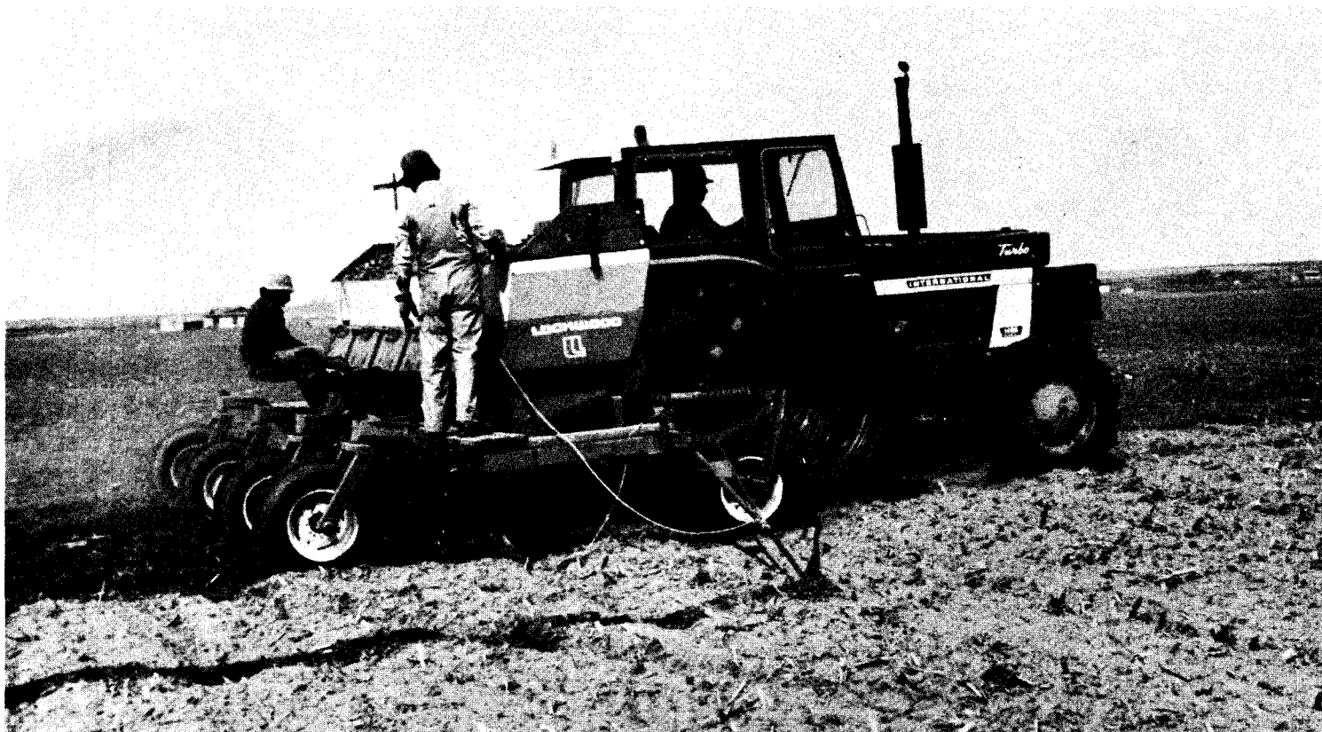
Fig. 13. Semi-mounted potato planters are used widely. Potato planters come in 2, 4, 6 or 8-row units. Picker arm and cup-type planters are the most popular.
